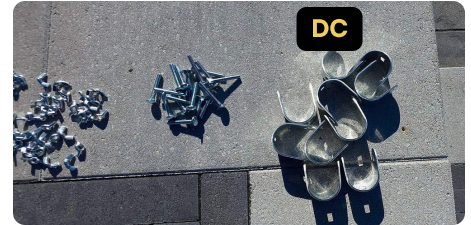
Hardware: wing nuts, bolts and half-collars DC
